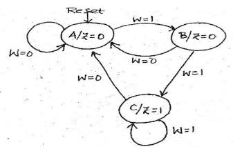
Design it using one-hot state assignment and implement it using Programmable Array Logic (PAL). (Apr 2017)
