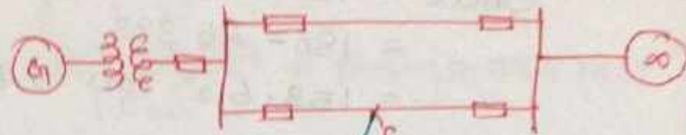
Fig: one machine system connected to a bus three phase fault @ 'F'.
